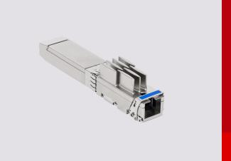
Ciena's Tibit™ MicroPlug™ OLT is a configurable ITU-T XGS-PON or IEEE 10G E-PON hot-pluggable SFP+ optical transceiver with a built-in 10G Ethernet-to-PON MAC bridge. It uses 10G XGS/10GE-PON optics to enable 10G PON solutions at a fraction of the cost of fixed-format OLT chassis and pizza boxes.
