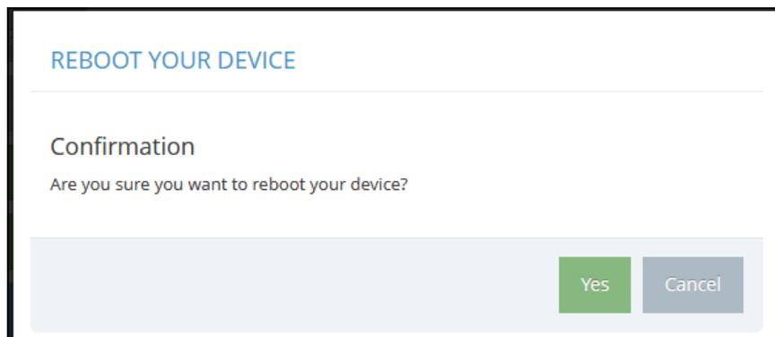
**Resetting the Access Point** The Reset page allows you to reset the access point to the factory defaults. Note that all user configured information will be lost. You will have to re-enter the default user name and password to re-gain management access to this device.
